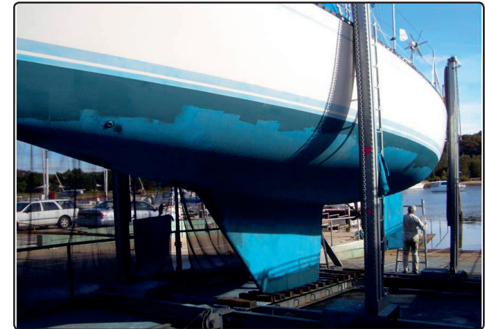
Water blasting showing removal of hydrolysed layers. Photo: Carboline
